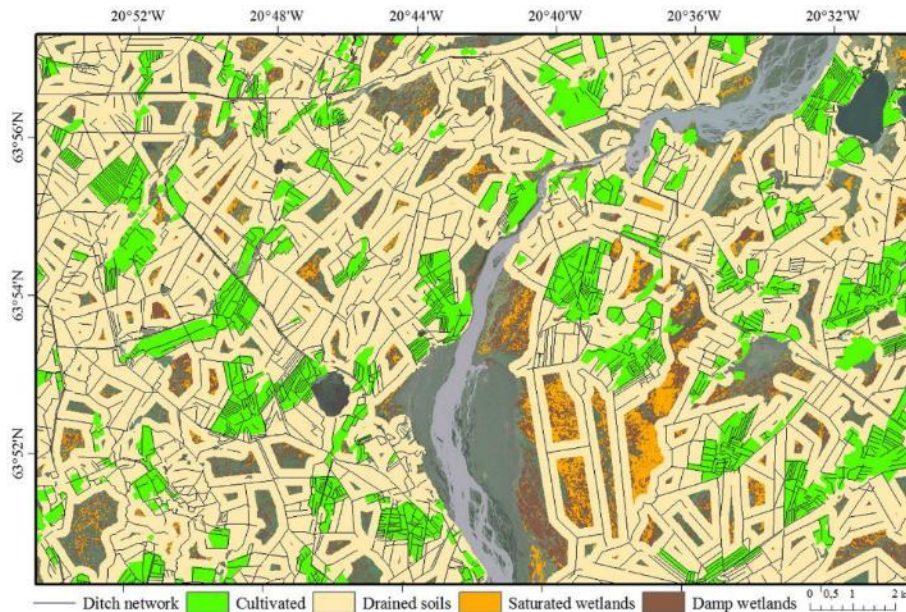
Figure A6.4 South Iceland, close to the river Þjórsá. The black lines show the system of ditches created to drain the wetlands. Of the drained soils, only the green patches are cultivated as hay fields (Arnalds, Gudmundsson, Oskarsson, Brink, & Gísladóttir, 2016).
