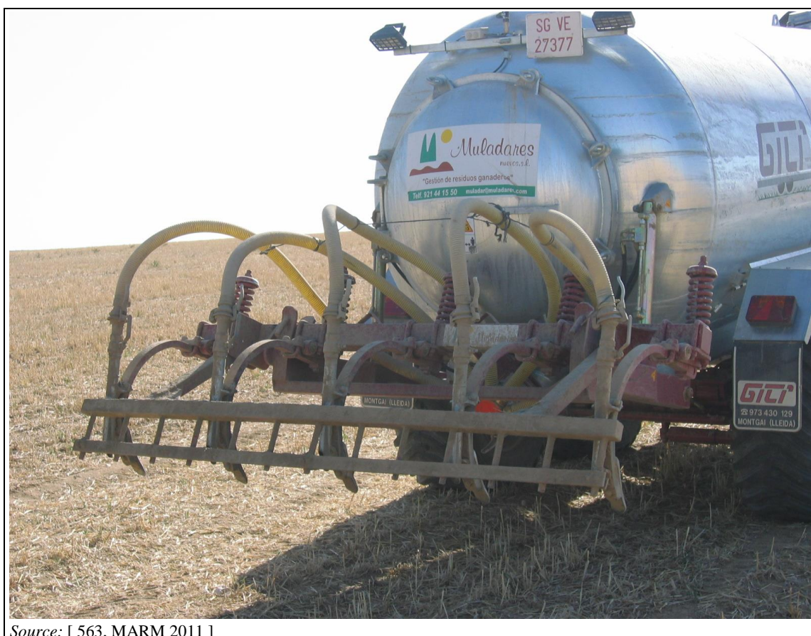
Figure 2.38: Example of an open slot injector
