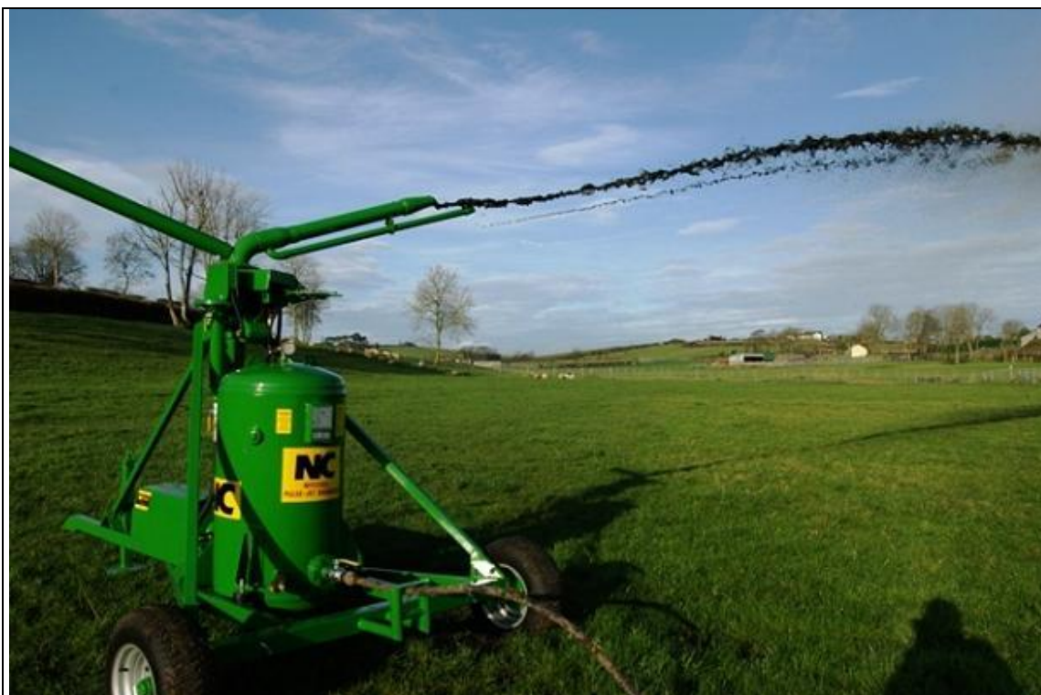
Figure 4.96: Pulse-jet irrigator in operation
