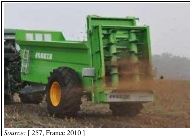
Figure 2.42: Vertical drum manure spreader
