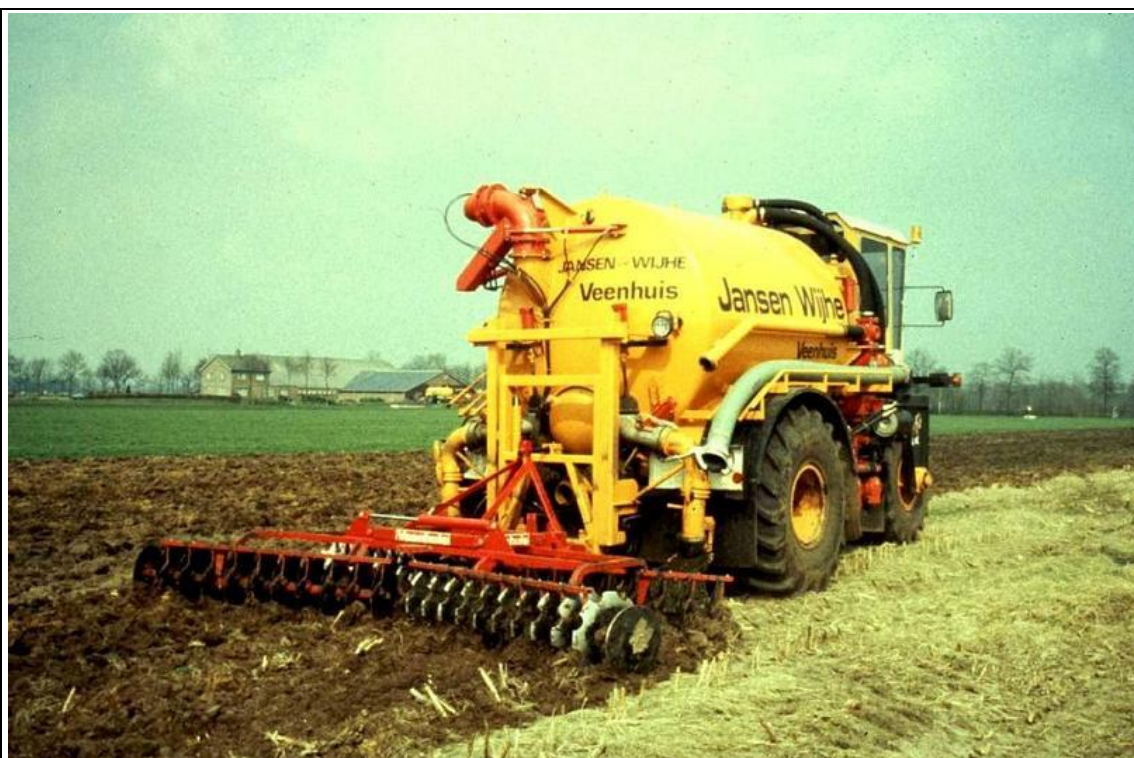
Figure 4.101: Incorporation equipment combined with a big tanker
