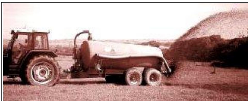
Figure 2.31: Example of a broadcast spreader with a splash plate
