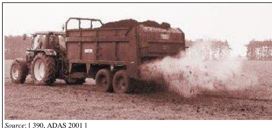
Figure 2.40: Example of a rear discharge spreader
