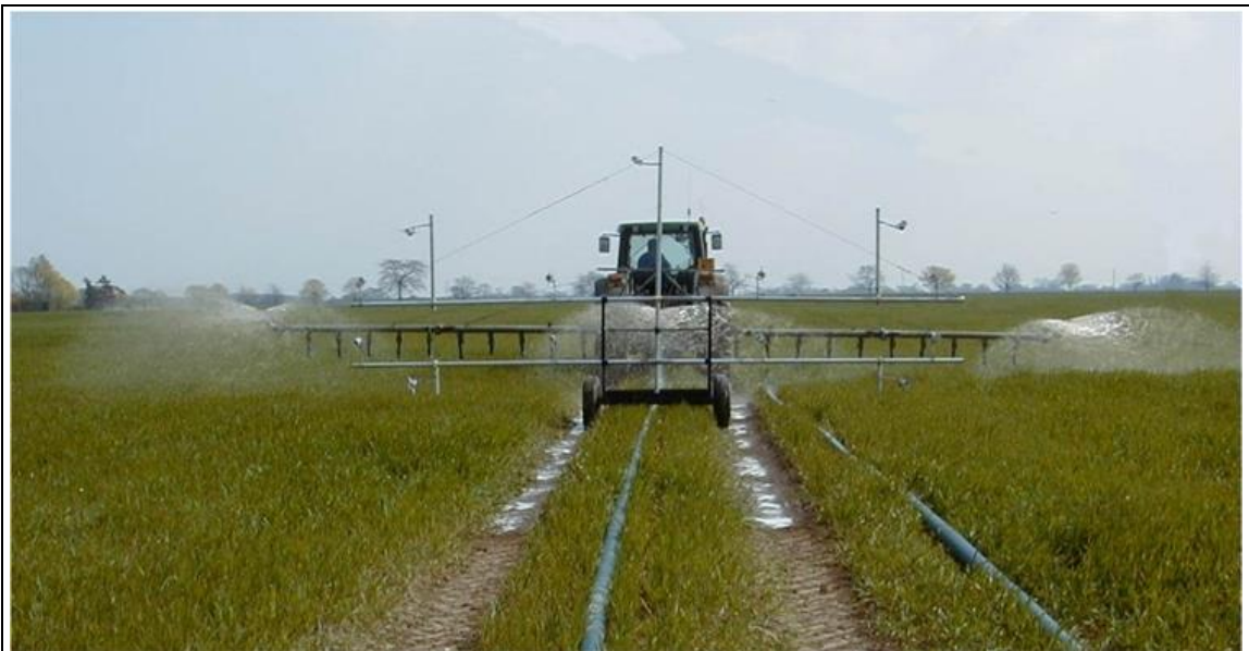
Figure 2.35: Rear view of a horizontal boom with splash plate for slurry application
